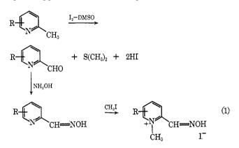
The 2 picolines were treated with 1 equiv of iodine at room temperature to form a crystalline complex which was dissolved in DMSO. The solution was heated to  $140-160^\circ$ ; a vigorous exothermic reaction occurred and dimethyl sulfide was evolved. After neutralization with aqueous alkali, the aldehydes were extracted and purified, or oximated directly. The aldoximes were treated with methyl iodide to form pyridinealdoxime methiodides as candidate enzyme reactivators.
